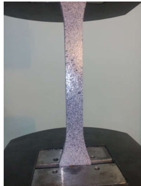
Figure 2. Tensile specimen clamped in tensile machine
